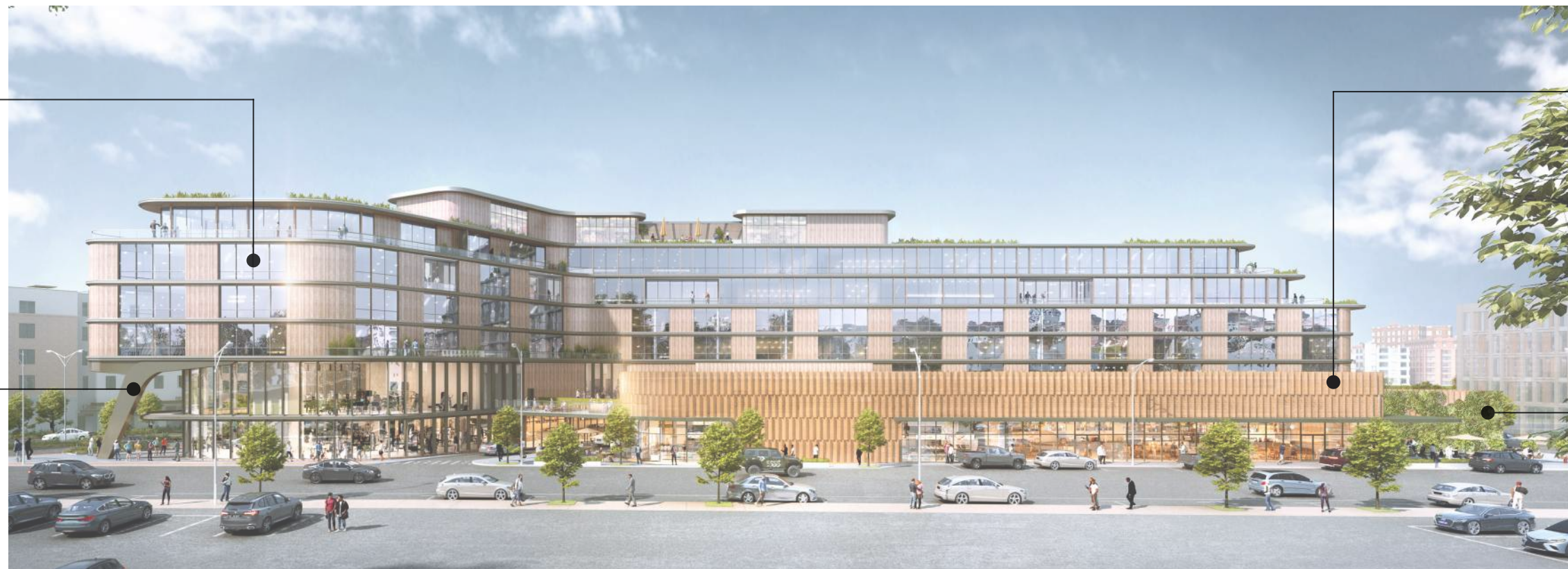
CONCAVE BRONZE PERFORATED AND SOLID METAL PANELS
