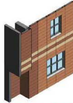
Terra Cotta Rain Screen Typical Assembly
